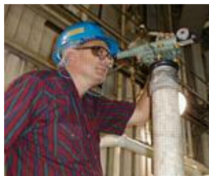
Optical measurement of thermal growth using a precision level
