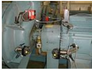
Permalign and Rotalign Pro M3 system measuring thermal growth; Agricultural Products Manufacturer in Nebraska.
